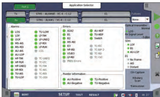
Quick overview of errors and alarms for both sides of SDH/SONET line
